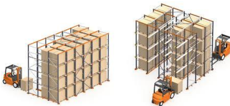
Figura 7: Sistema Drive-In (à esquerda) e Drive-Through (à direita). Fonte: https://www.interlakemecalux.com/storage-racks/drive-in-drive-thru-pallet-racks
