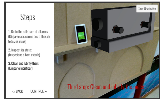
Figure 6: System UI/UX for maintenance procedure.
