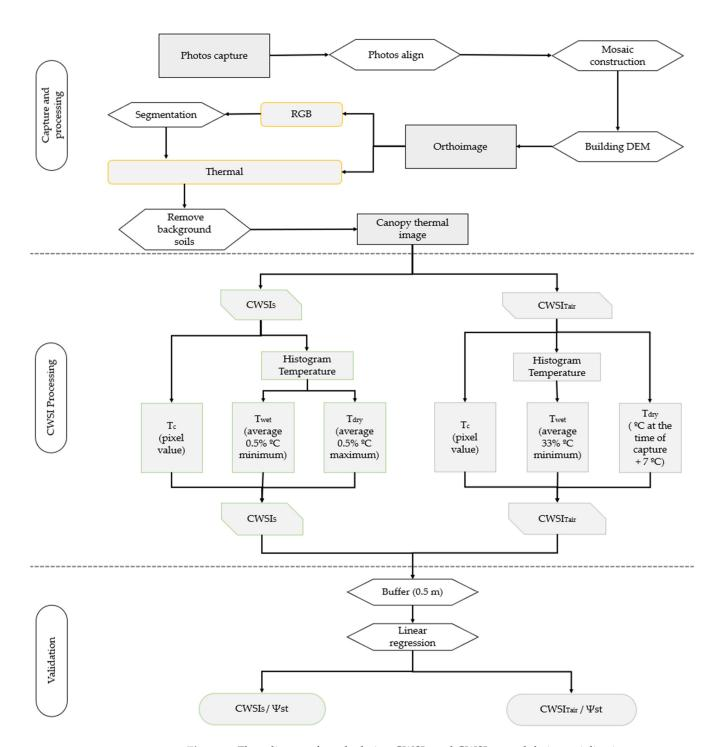
Figure 2. Flow diagram for calculating  $\mbox{CWSI}_S$  and  $\mbox{CWSI}_{\mbox{Tair}}$  and their spatialization.
