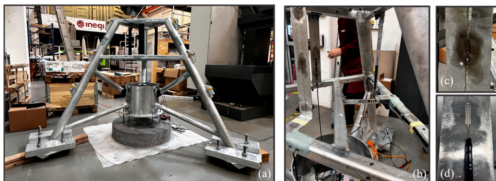
Figure 3. Final structure. (a) Overall lander structure; (b) specific plates mounted on the structure where strain gauges are mounted; (c) primary system—optical strain gauges' assembly; (d) secondary system—electrical strain gauges' assembly.
